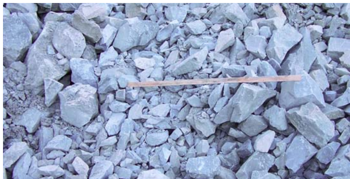
Rocklock delivered a higher degree of fragmented rock with a more uniform size distribution
